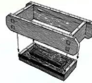
Shaping moulding of the bricks by hand
