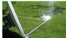
Mirror pieces will converge the sunlight to one point
