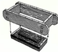
Shaping moulding of the bricks by hand
