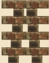
Perforated wall made by bricks.
